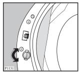
When the appliance is to be scrapped, cut off the electrical supply cable and destroy the plug with the remaining cable. Disable the door catch in order to prevent children from becoming trapped inside while playing.
